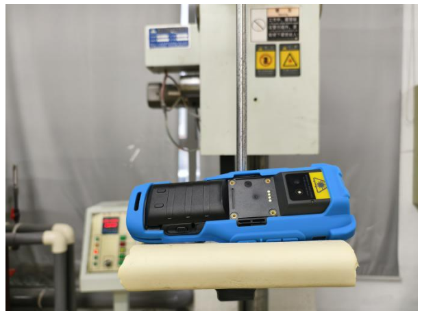
In Testing (edge 12)
